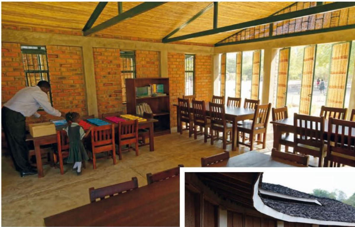
ABOVE & RIGHT: Features such as woven screens at Lupani Community School and the curvature of the building at Ilima Primary School help circulate air in hot climates such as Zambia and the Democratic Republic of Congo, respectively.
