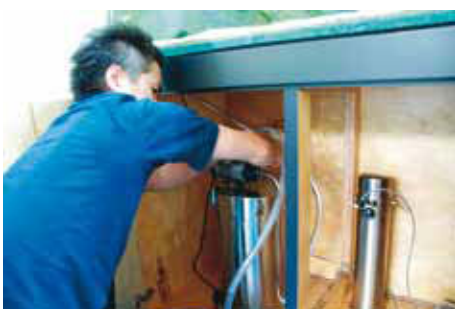
The Wood Cabinet is installed with an ADA CO2 Tower and two ADA Super Jet Filter ES-2400.
