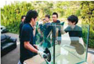
Suckers are attached to the side of the aquarium to make it easier to move. These are an indispensable piece of equipment.
