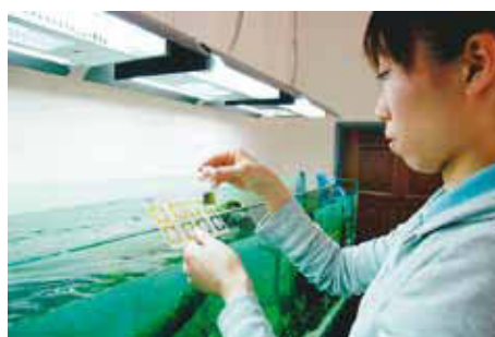
One week after the set up, because we are using filter medium that has already been matured in another tank in advance, there is no occurrence of ammonia.
