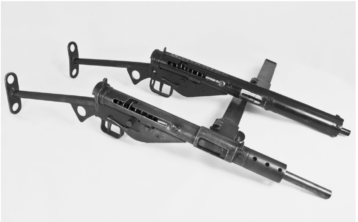
27. Mk II (bottom) and Mk III (top) Sten guns, 9mm calibre. Effective range 110 yards (100m); weight 3.2kg (7.1lb). Began to be issued to the Auxiliary Units in September 1942. The main virtue of the Sten gun was that it was cheap to manufacture, but it had a poor reputation for reliability. It was well designed for clandestine warfare as the horizontal magazine (32 rounds) allowed it to be easily fired from prone position. (© Kate Atkin)
