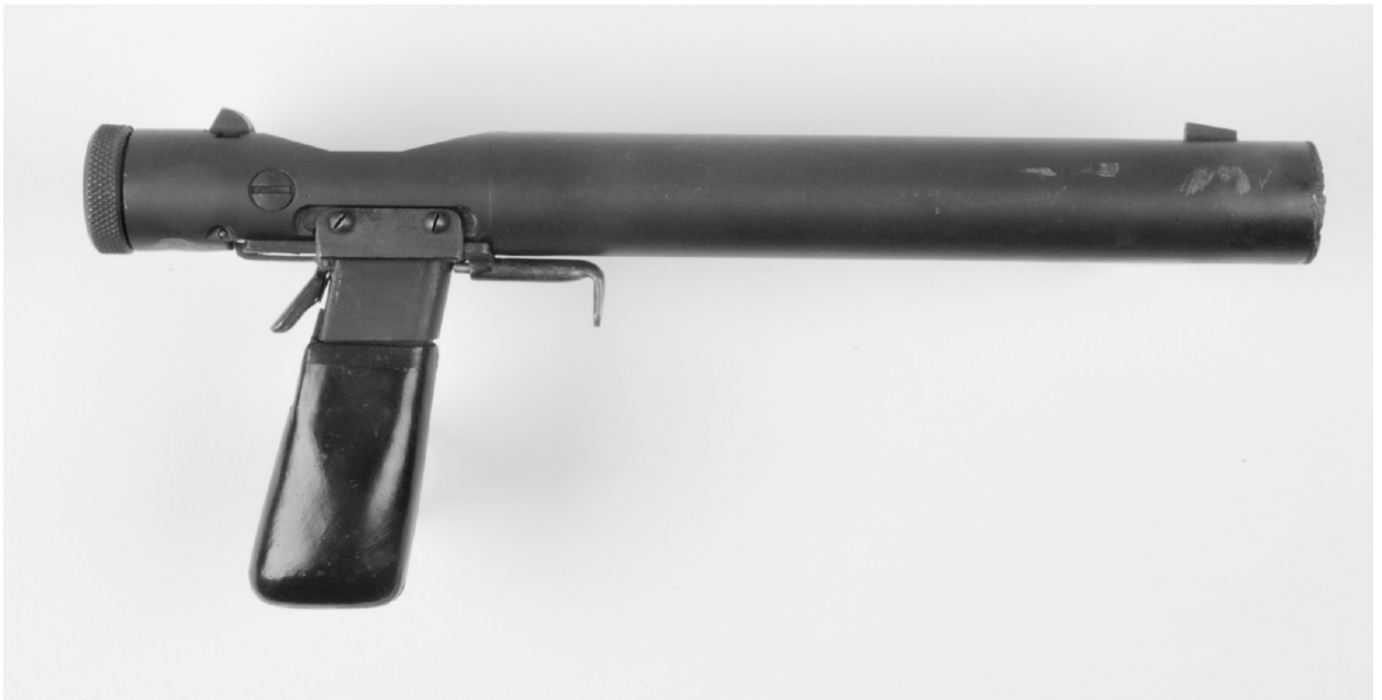
23. Welrod bolt-action silenced pistol with 8-round magazine, .32 Calibre. Range point-blank to approximately 23m. It requires a two-handed grip to control properly. (© Imperial War Museums, FIR 2979)
