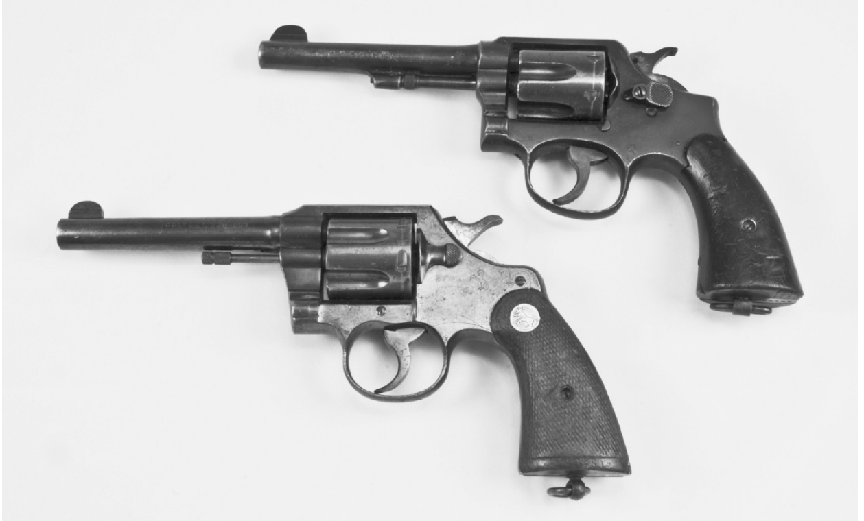
22. Smith and Wesson Model 10 (top) and Colt New Service .38 (bottom) revolvers as issued to the HDS and Auxiliary Units. Many were ex-US police issue. (© Kate Atkin)
