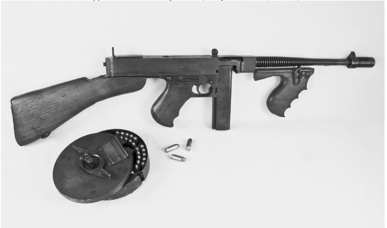
26. Thompson M1928A1 sub-machine gun.45ACP calibre. Effective range 55 yards (50m); weight 4.9kg (10.8lb). This example has a simplified rear sight. Although most Thompsons were replaced in the Auxiliary Units by Sten guns during 1942, some remained in use until October 1943. The impressive-looking drum magazines contained 50 rounds but were heavy, rattled and took a long time to reload. The stick magazines containing 20 rounds were usually preferred. (© Kate Atkin)
