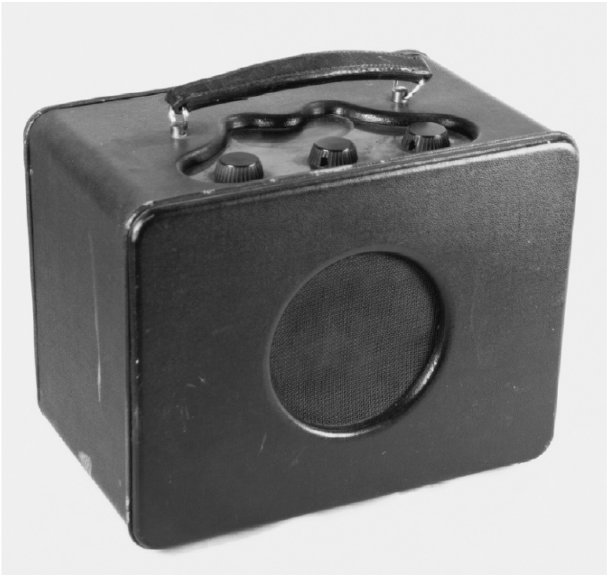
34. Murphy B81 portable battery-powered wireless (1939). This became a standard issue to the military, including the SDB, to receive the BEETLE emergency broadcasts. (© Susanne Atkin)
