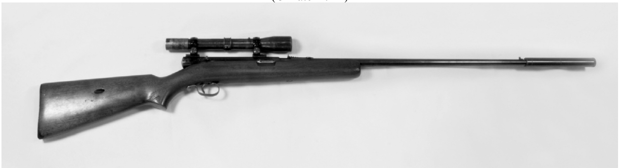
28. Winchester 74 sniper rifle of the type issued to the Auxiliary Units, .22L Calibre. Effective range 100 yards (91m). These civilian rifles were fitted with sound moderators and most had telescopic sights, although the latter were considered unsatisfactory by the Auxiliary Units Training Officer, Nigel Oxenden, as they kept going out of alignment and had to be adjusted by armourers. Remington and Martini models were also used by the HDS and Auxiliary Units, but the semiautomatic Winchester 74, issued from 1942, was particularly silent in operation as it had a closed bolt. It was also issued to SOE. (© Kate Atkin)
