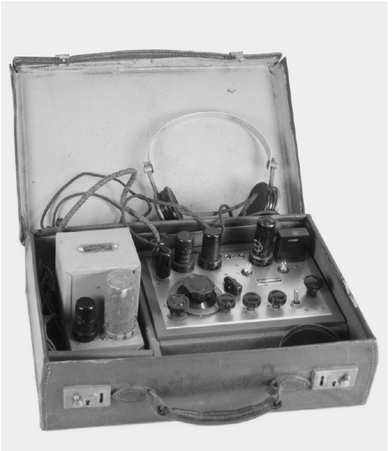
37. SIS Mk VII 'Paraset' transceiver (replica by Malcolm Atkin). A 'suitcase' set used as backup set by SCUs and possibly by Eastbourne Section VII cell from 1941. (© Susanne Atkin)
