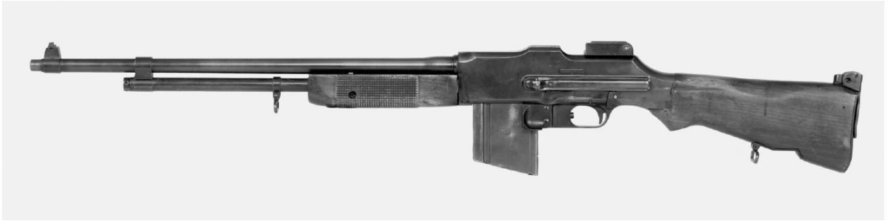
25. M1918 Browning Automatic Rifle (BAR), 7.27 kg, .30-06 calibre. Effective range up to 1,500 yards (1370m); weight 7.27kg (15.98lb). Too cumbersome for patrol work but the earliest automatic weapon supplied to the Auxiliary Units. (© Royal Armouries, PR.5306)
