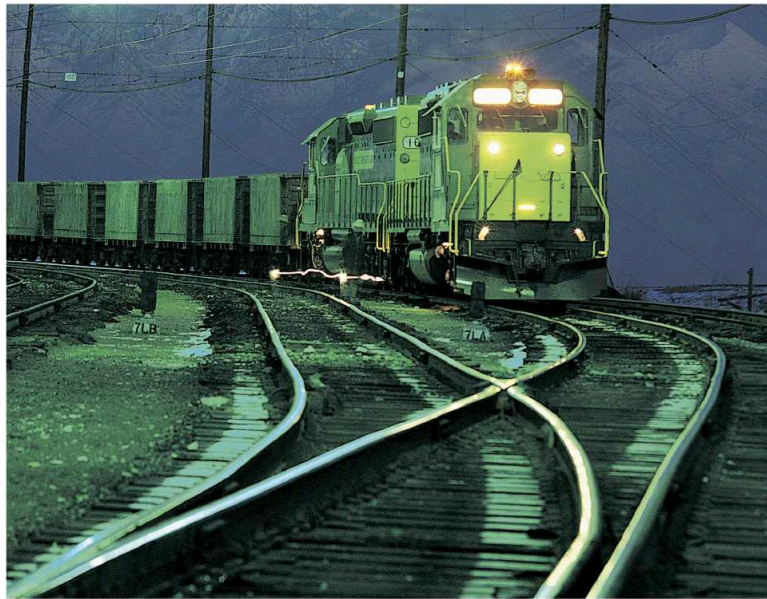
A FREIGHT TRAIN WAITS ON A SIDING, LEAVING THE MAIN LINE UNOBSTRUCTED
