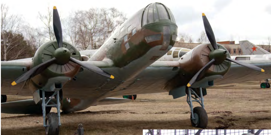
Left: DB-3 – the first Soviet long-range bomber developed under the direction of Sergey Ilyushin. Batch production started in 1936 and a total of 6,735 of all versions were built, including the DB-3F (Il-4). It was using the DB-3Fs that the Baltic Fleet’s 15 crews made the first bombing raid on Berlin on the night of August 8, 1941.
