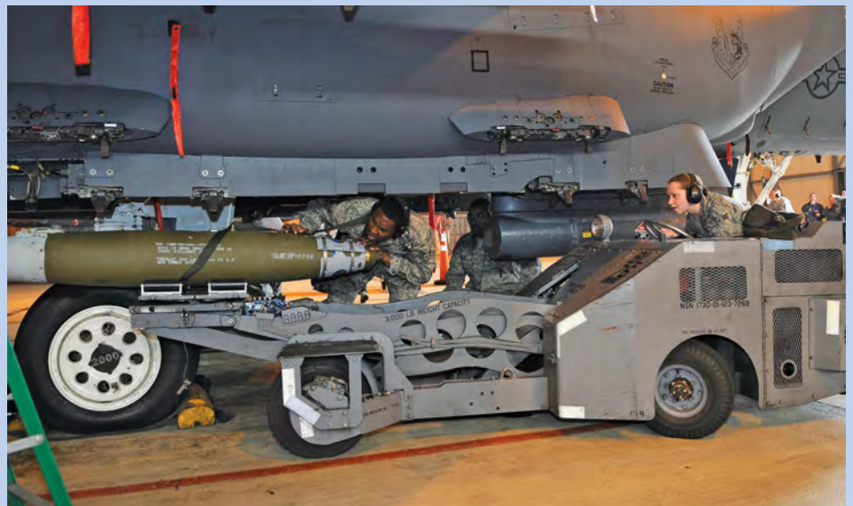
Above: A GBU-38 JDAM is loaded onto an F-15E at RAF Lakenheath. USAF/Staff Sgt Connor Estes
