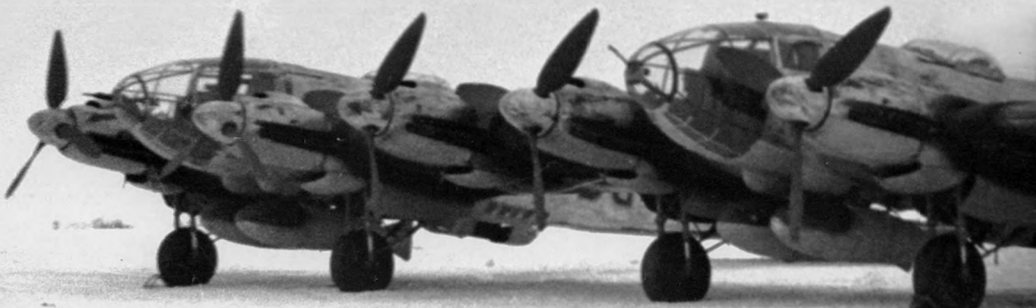
Below: An He 111 Z-1 of GS-Kommando 2 in the Crimea in early 1943. The aircraft was used to tow the Me 321 Gigant glider. EN-Archive
