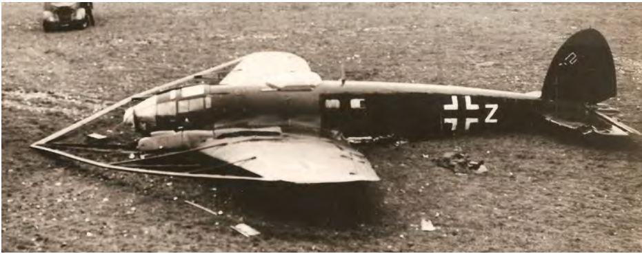
Above: This He 111 H-8, Werk Nummer 3944 coded 1G+ZM of 4/KG 27, crash-landed at Lulworth, Dorset on May 22, 1941. The Kuto-Nase barrage balloon cable cutter was of particular interest to the RAF. Chris Goss Collection
