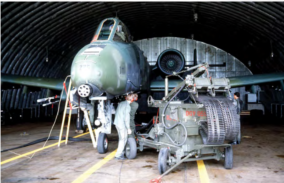
Above: Ground crew load a GAU-8 Avenger at Ahlhorn in West Germany. The detached flights conducted live fire exercises at the Grafenwöhr or Hohenfels ranges in Bavaria. USAF
