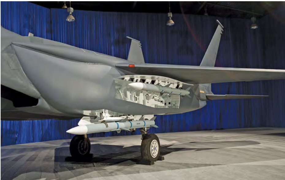
A close-up view of the new conformal weapons bays on the F-15SE. Boeing
