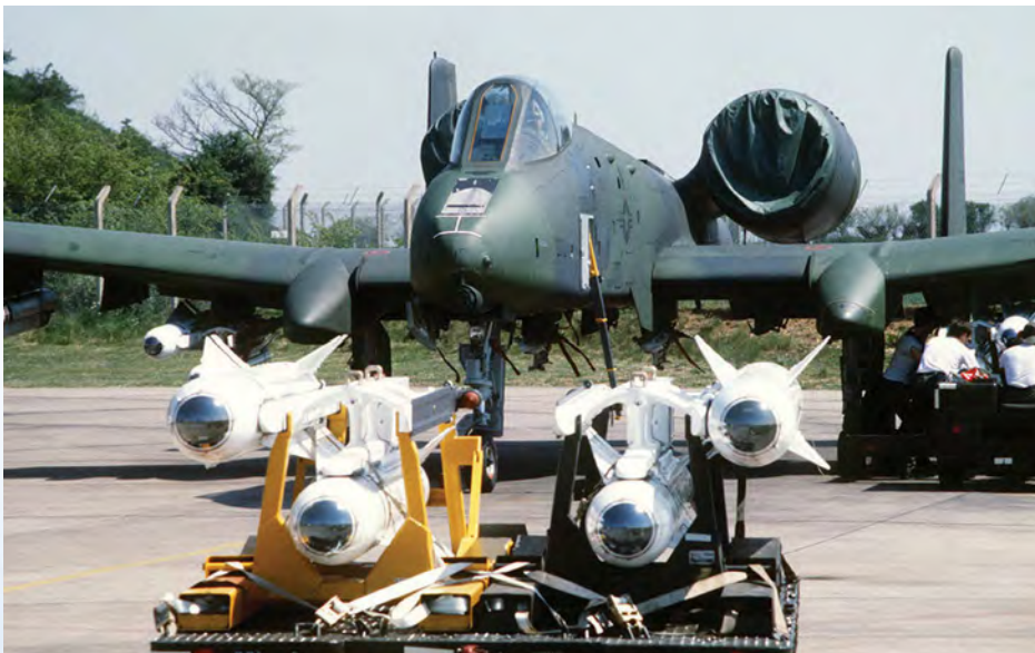
Below: An A-10 awaits the mounting of four Maverick missiles at RAF Bentwaters. USAF
