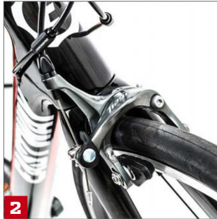
1 On to the R4's full-carbon frame are bolted an aluminium seatpost, bars and stem from Ritchey 2 Continental tyres provide a good balance of rolling resistance and grip while Tiagra callipers control your speed 3 The drivetrain comes in the shape of a full 10-speed Tiagra groupset but would benefit from an 11-tooth sprocket
