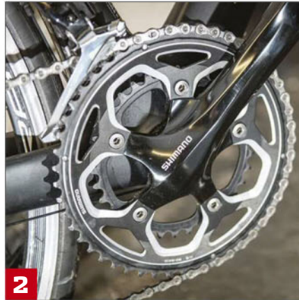
1 Shimano's 105 components make up much of the Ridley's groupset and provide crisp shifting 2 A 50/34-tooth chainring encourages you to spin the pedals rather than grind them round, and save more of your leg strength for the run 3 4ZA's stub-nosed saddle provides plenty of cushioning while allowing you to roll forward into a tuck
