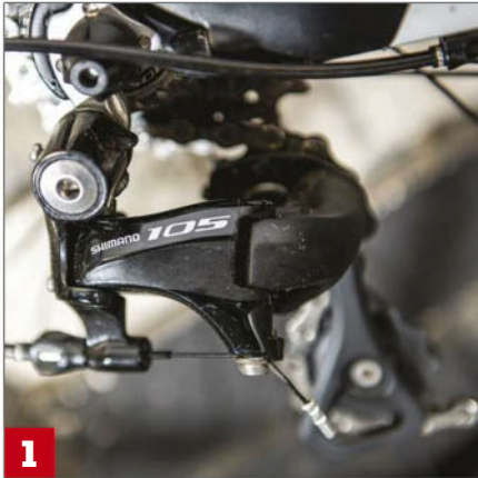
1 Shimano's 105 components make up much of the Ridley's groupset and provide crisp shifting 2 A 50/34-tooth chainring encourages you to spin the pedals rather than grind them round, and save more of your leg strength for the run 3 4ZA's stub-nosed saddle provides plenty of cushioning while allowing you to roll forward into a tuck
