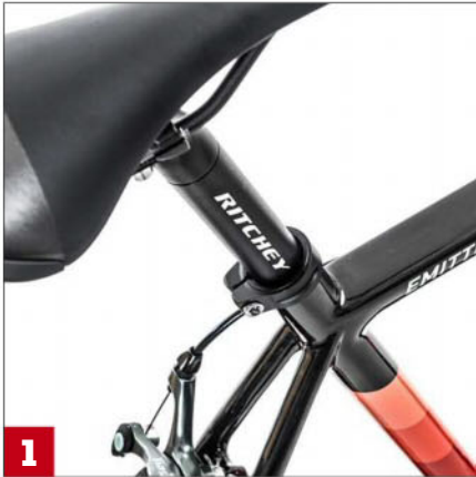
1 On to the R4's full-carbon frame are bolted an aluminium seatpost, bars and stem from Ritchey 2 Continental tyres provide a good balance of rolling resistance and grip while Tiagra callipers control your speed 3 The drivetrain comes in the shape of a full 10-speed Tiagra groupset but would benefit from an 11-tooth sprocket
