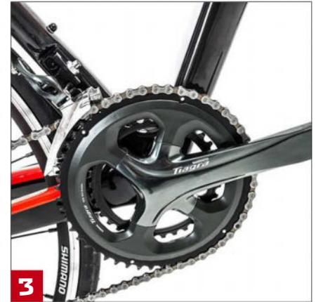
1 On to the R4's full-carbon frame are bolted an aluminium seatpost, bars and stem from Ritchey 2 Continental tyres provide a good balance of rolling resistance and grip while Tiagra callipers control your speed 3 The drivetrain comes in the shape of a full 10-speed Tiagra groupset but would benefit from an 11-tooth sprocket
