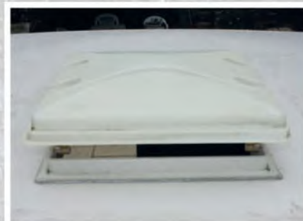
Next, carefully place the pop-up unit covers back into their original position
