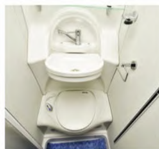
Corner washroom has tip-up basin above a bench toilet
