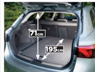
The rear seats fold almost flat to yield a well-shaped load bay BELOW Boot space is average
