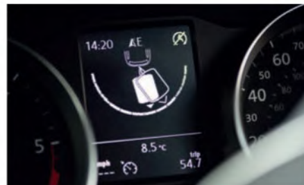
It determines the van's wheelbase by noting the angle of the hitch at the start of the turn
