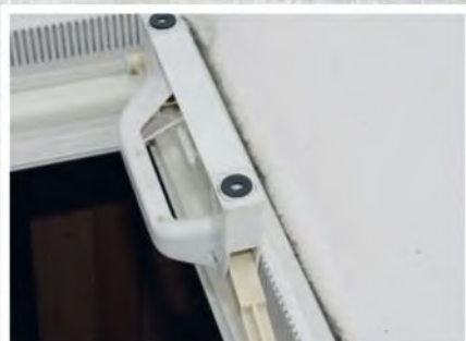
Ensure that the black rubber washers are correctly seated — these form the main seal
