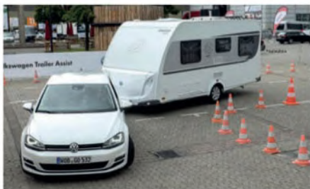
The driver uses the door mirror adjuster to pick the angle and direction of the turn
