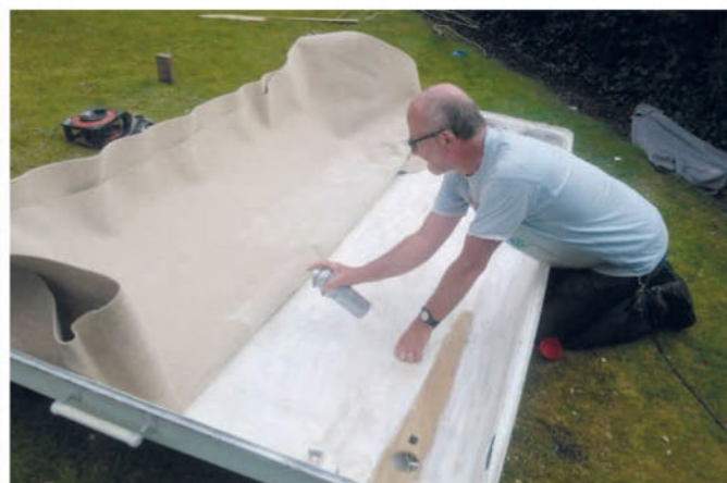
Repairs to the Portafold were cosmetic rather than structural. Here, Jeremy replaces the roof lining with headlining material in Ventrup
