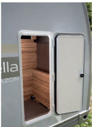
ABOVE The large external locker takes up the kitchen's dead space RIGHT Gas locker holds other kit. You can stand on the long A-frame
