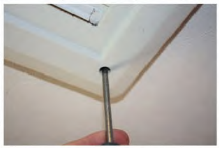
Remove the screw caps from the inner trim, then the screws that secure the latter
