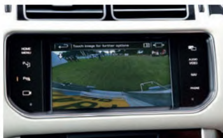
The cameras send images that combine to give the impression there is no caravan
