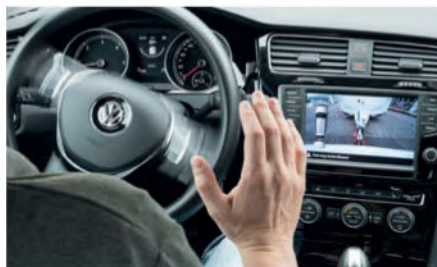
The system helps steer the car through the manoeuvre while the driver controls speed
