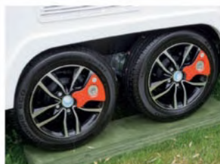
The grabhandles have LED courtesy lights behind them to make finding them at night simple RIGHT The alloy wheels get AI-Ko Secure locks
