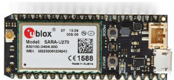
Above The Electron Particle 3G comes with its own SIM card and a plug-in system for extensions
