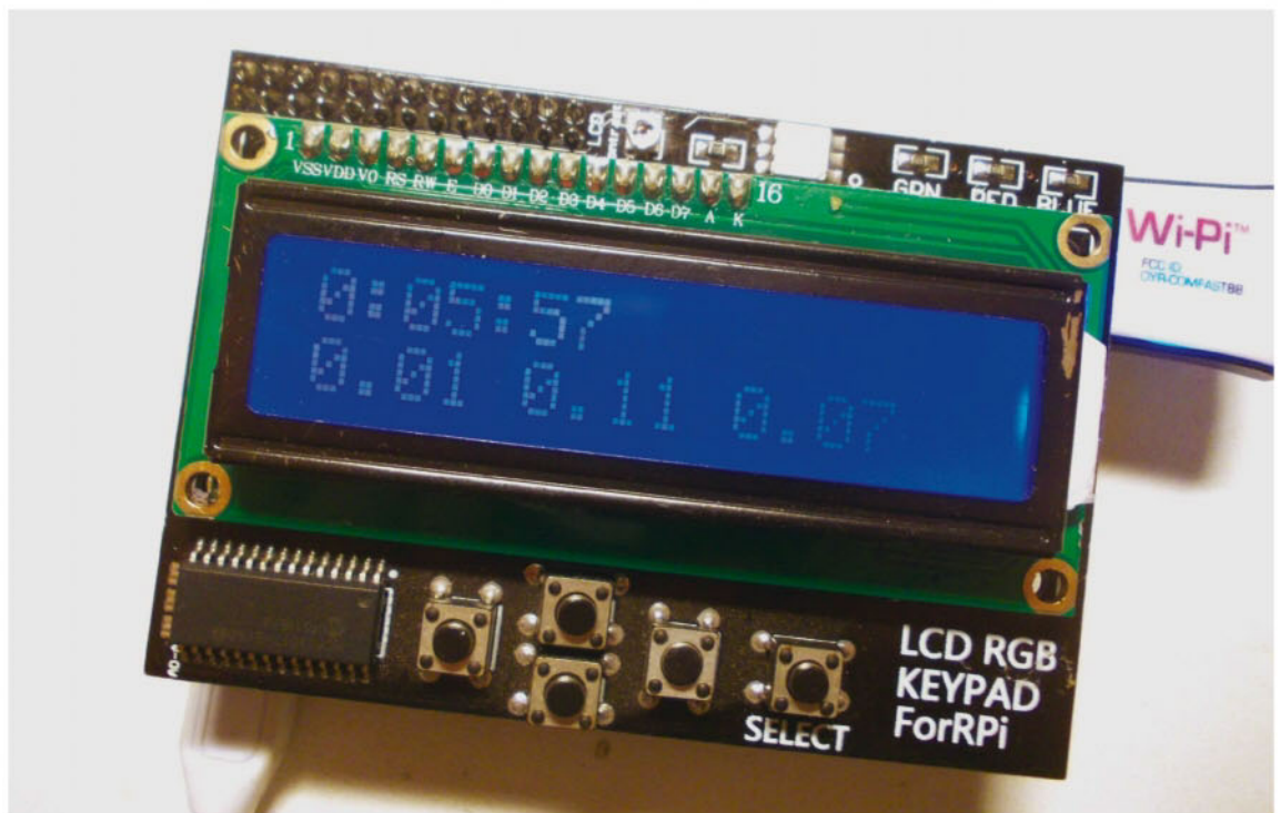
Above With a couple of button presses, you can monitor your system parameters with pyLCl
