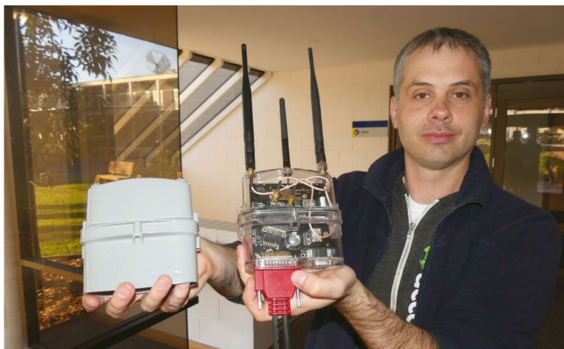
Above The newly manufacturable Serval Mesh Extenders are used to connect communities together without the need for a cellular tower
