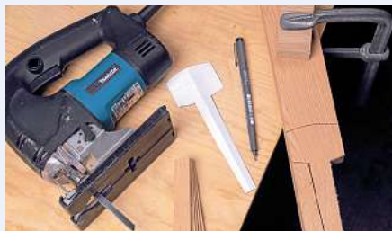
Clamp several layers of wood together tightly.
