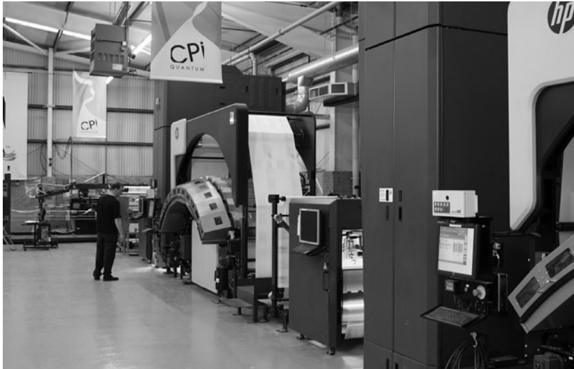
CPI Group's first colour Quantum, installed at Antony Rowe in Chippenham in 2012: an HP T360 inkjet press coupled with a Timson T Fold finishing line
