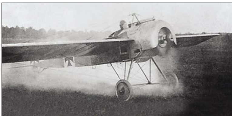
Above: The pilot opens up his aeroplane's 100hp Oberursel rotary engine as he heads off for another mission over the front line in his Fokker E.III. via Aviation-images.com
