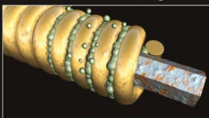
Gaps between the windings are not protected
