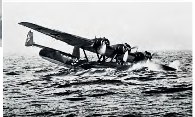
Making a splash. This Do 24K-2 has just landed in rough seas and shows how effective the fuselage side floats were to keep the aircraft afloat. EN Archive
