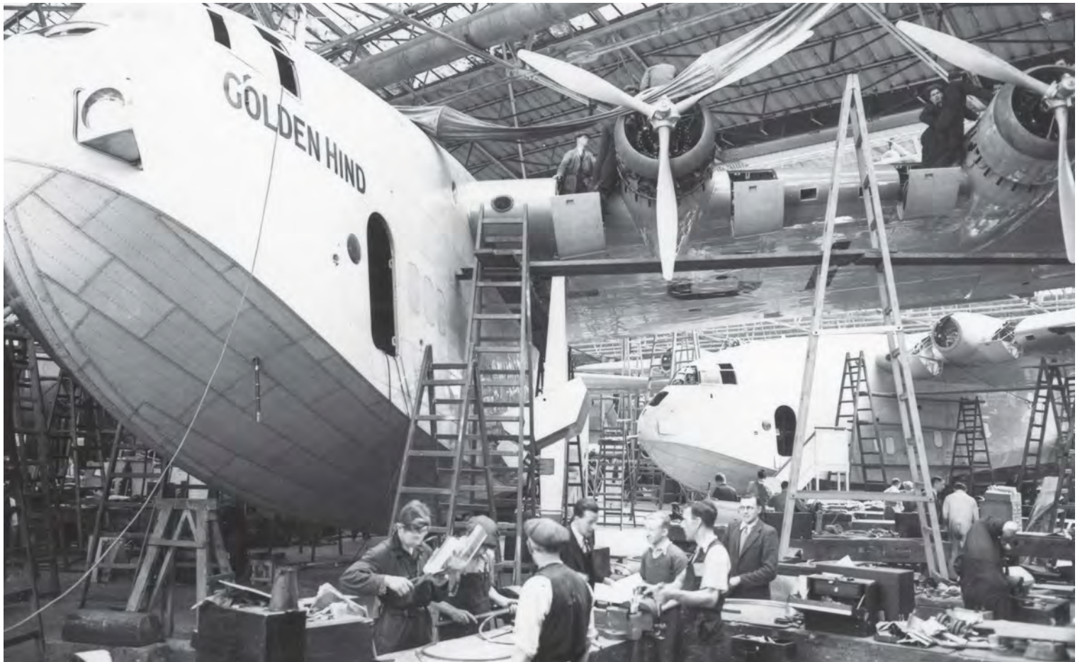
Two of the majestic Short 'G' Class flying boats nearing completion at Rochester. Originally intended for transporting up to 2 tons of mail over distances up to 2,500 miles, the three completed 'G' Class Empires were quickly impressed into military service and militarised with defensive turrets.
