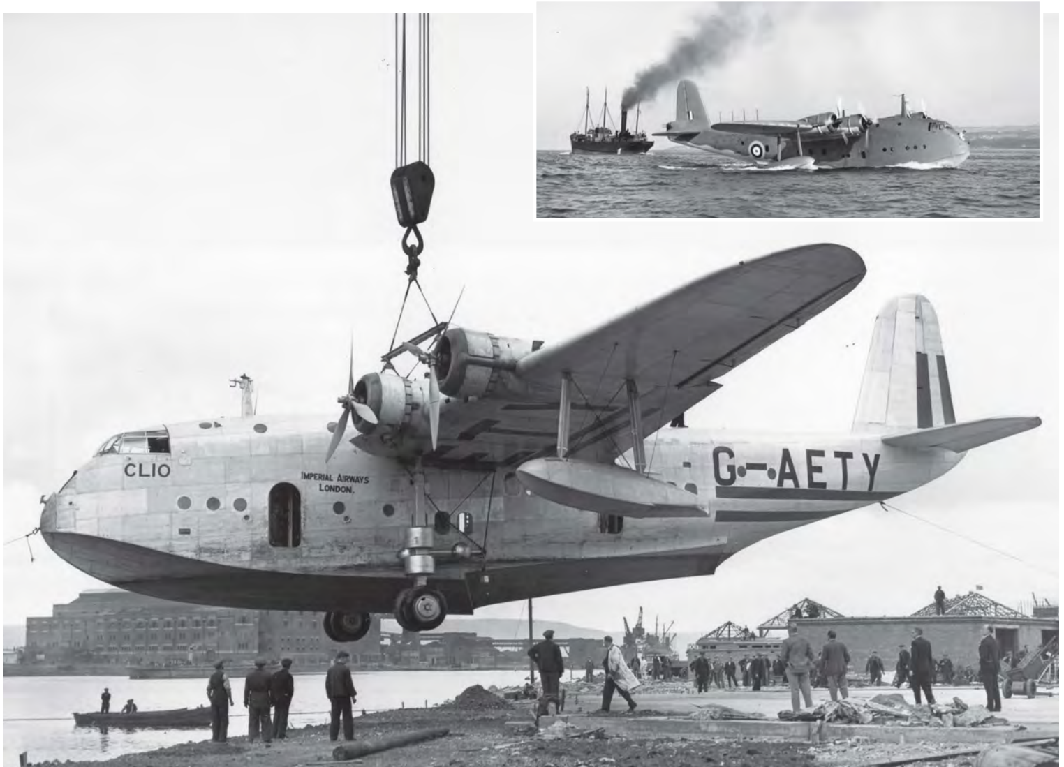
Short 'C' Class S.23 Clio flying boat before and after militarisation. As AX659, Clio was fitted with ASV radar equipment (hence the proliferation of aerials over its rear fuselage) and defensive dorsal and tail turrets. The aircraft crashed into high ground near Bowmore, Loch Indaal, on 22 August 1921 after an engine failure.
