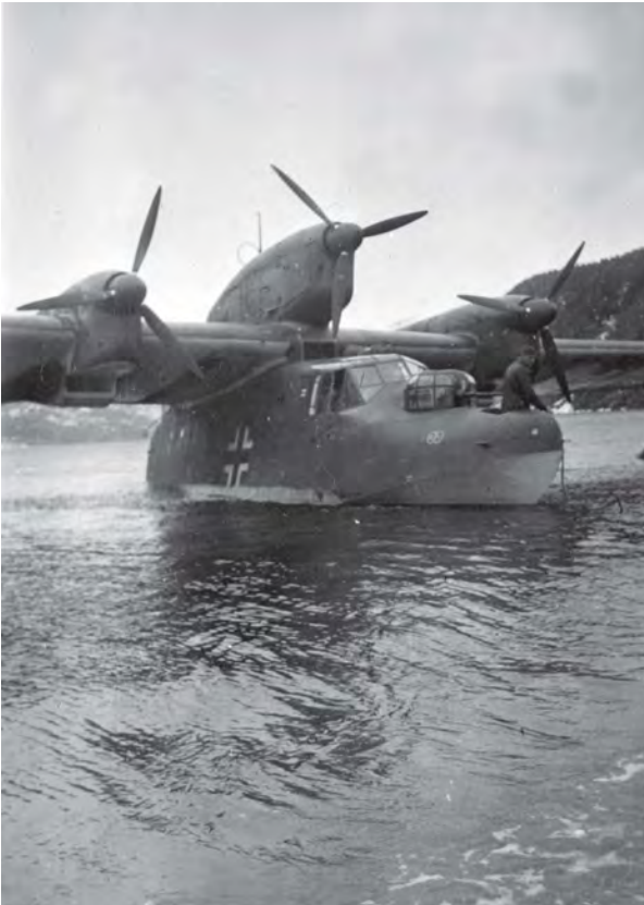
The unusual configuration of the BV138 is well shown by this shot taken at Hemnesfjorden, Norway, in May 1940. This is an early production aircraft featuring the three-bladed propeller on the middle engine.
