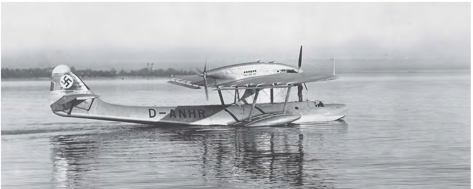
Record-breaking Dornier D-ANHR is reflected in the stillness of the water. This Do 18D was taken off the military production line and had its wingspan increased to establish a seaplane distance record of 5,219 miles in 1938.
