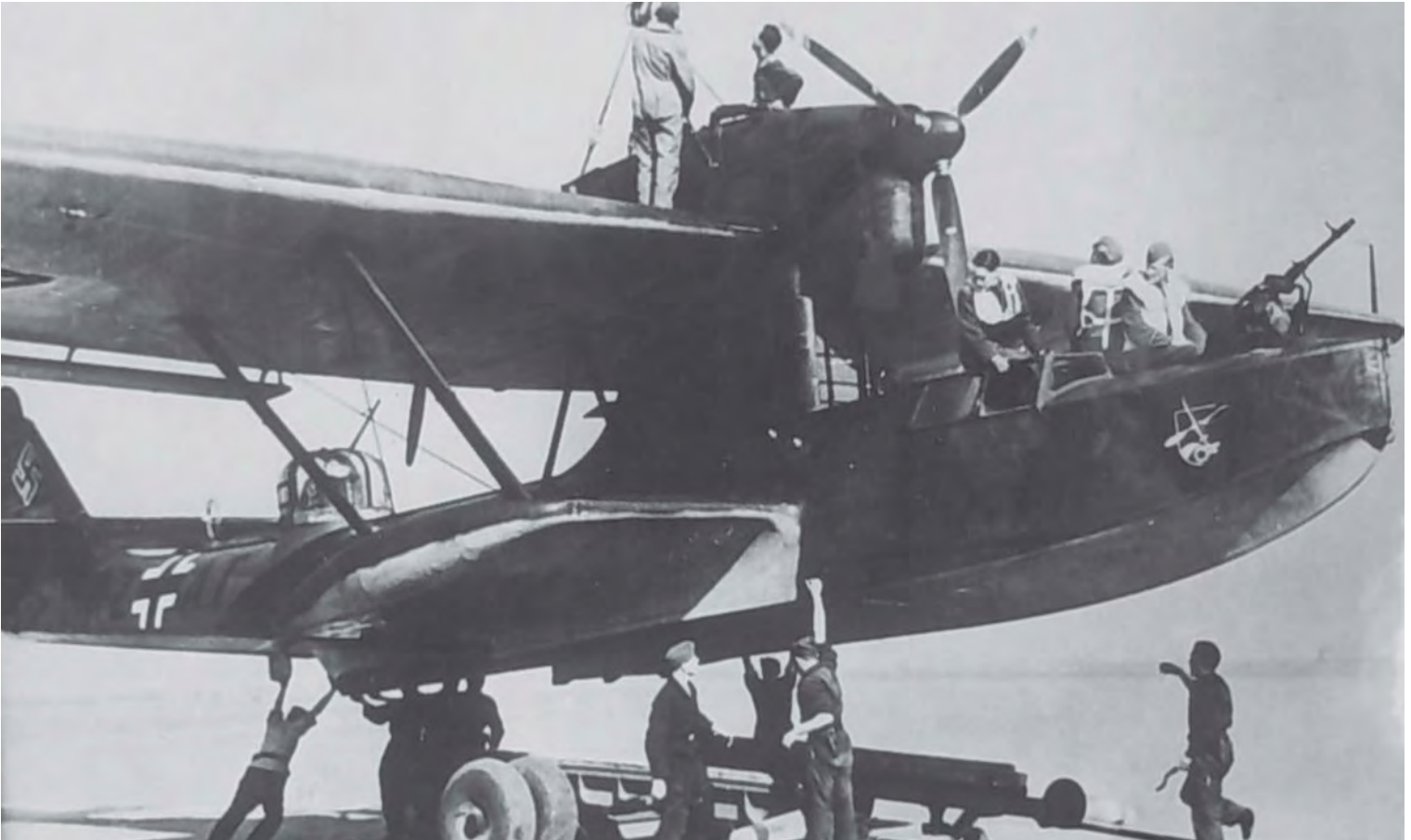
A Dornier Do 18G-1 on the French channel coast early in 1942. This version was armed with a power-operated dorsal turret.
