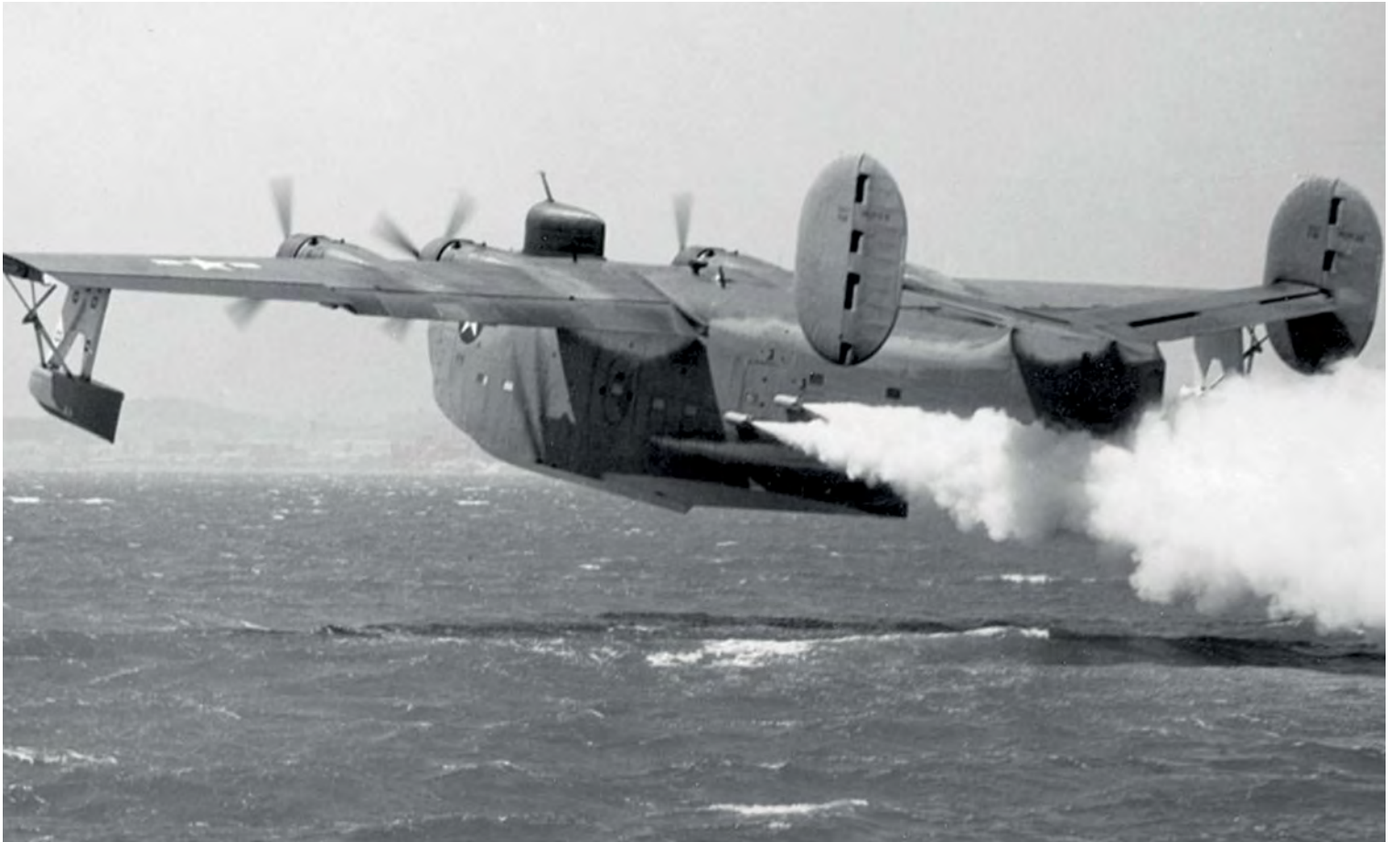
The performance of the Coronado PB2Y-5H was enhanced by JATO, jet assisted take-off rockets.
