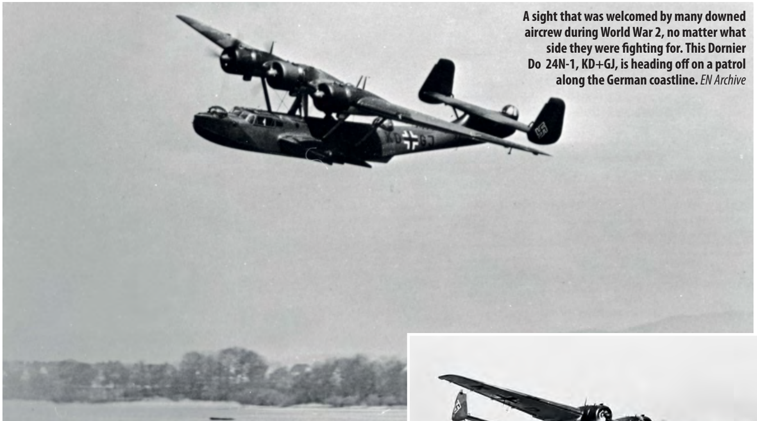
Making a splash. This Do 24K-2 has just landed in rough seas and shows how effective the fuselage side floats were to keep the aircraft afloat. EN Archive
