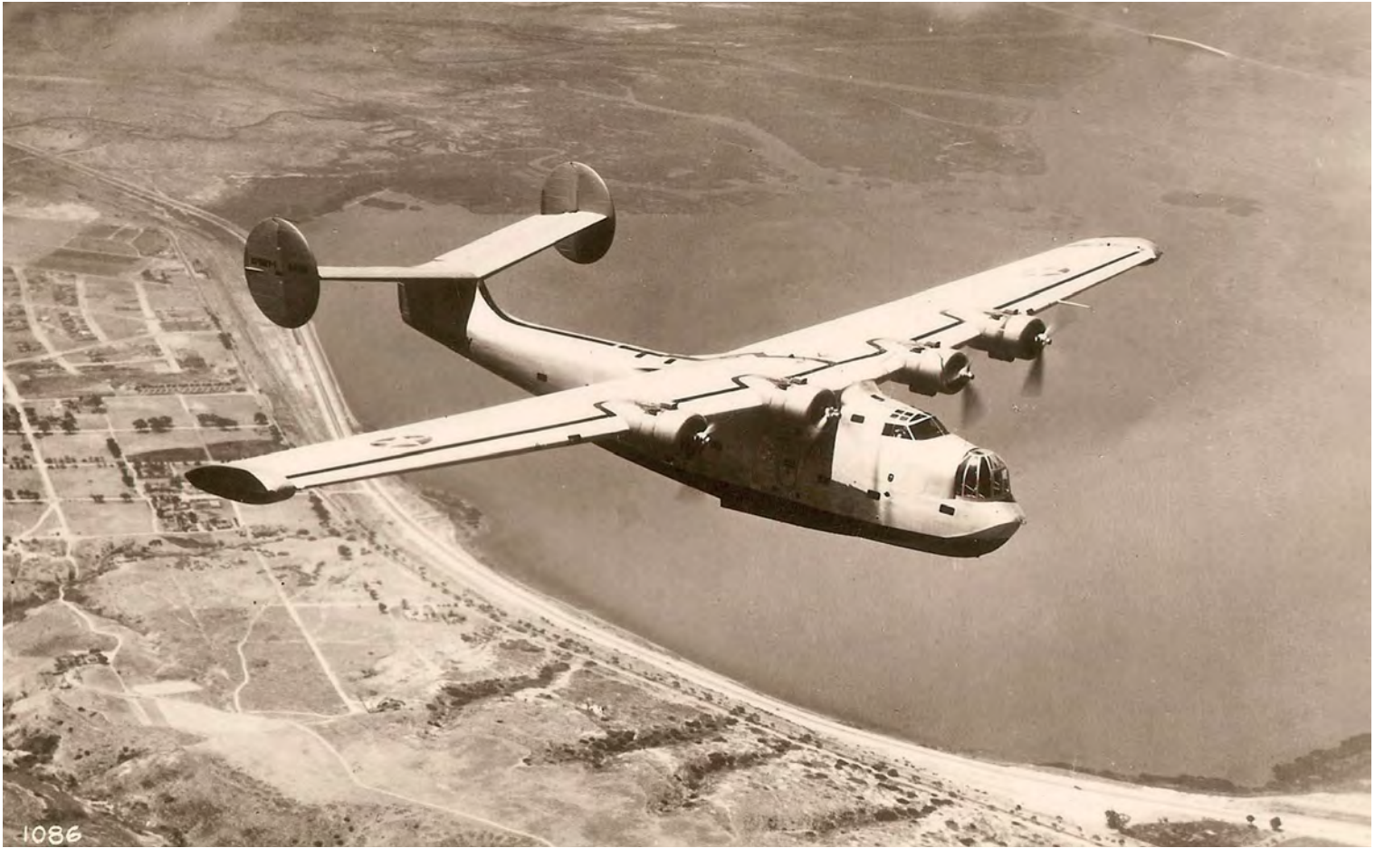
The XPB2Y-1 prototype Coronado in its third modification fitted with a redesigned twin tail section to improve lateral stability. The tail fins on this version were practically circular, whereas production models featured a more oblong design, similar to those of the B-24 Liberator.
