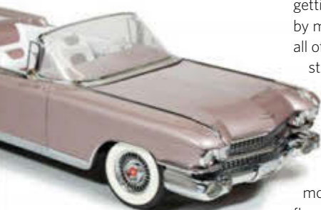
ABOVE The Cadillac was developed over the course of eight months, and created with the use of over 95 per cent 3D printed parts
