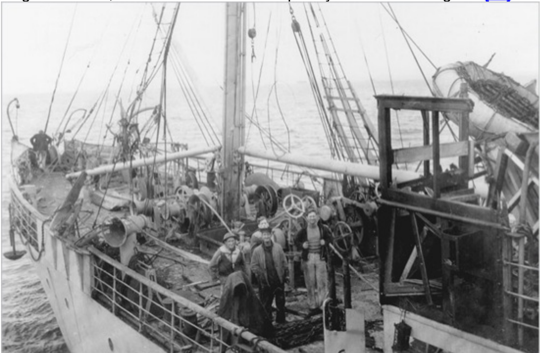
The damage to Monarch was extensive. The broken structure to the right of the photo is Monarch's bridge. The
