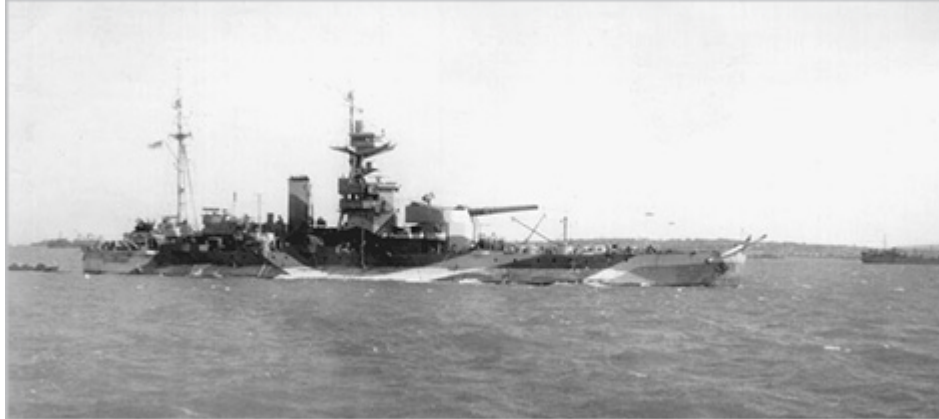
HMS Roberts classed as a monitor, on June 7, 1944. The ship is the size of a cruiser but mounted with a battleship turret. It is designed to anchor off-shore and bombard enemy positions with heavy fifteen-inch guns.
