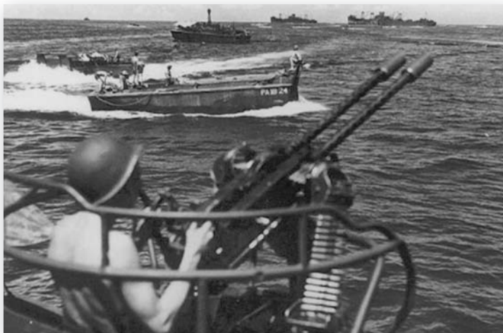
Here a PT boat escorts LCVP landing craft to shore providing antiaircraft protection. Most .50-cals dispensed with flash suppressors, but these guns had tube-type suppressors. Others had cone-shaped flash-hiders.
