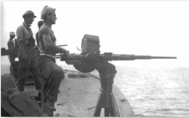
A boat's officer mans a 20mm Mk 4 cannon on a lightweight Mk 14 mount. These low mounts were less than effective for antiaircraft use, although they could be so employed, but the gunner was squatting on the deck. Such mounts were intended for surface targets.
