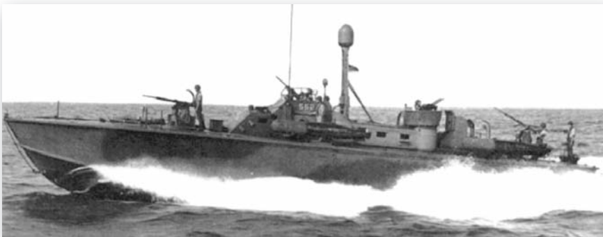
PT 552, a Higgins of the PT 486–563-class, has a second 20mm Mk 4 cannon mounted on the forecastle. The forward 20mm would have a lighter mount than its aft brother.
