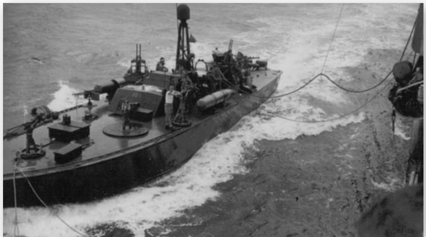
PT 191 replenishes fuel from a seaplane tender while underway. Seaplane tenders frequently serviced PT boats as they had aboard a significant aviation gasoline fuel store. Other boats are lined up awaiting their turn. This boat is armed with a 37mm M4 gun, a 20mm Mk 4 on the port beam, a twin .50-cal on the starboard beam, two Mk 13 torps, and a 40mm M1 gun on the fantail.
