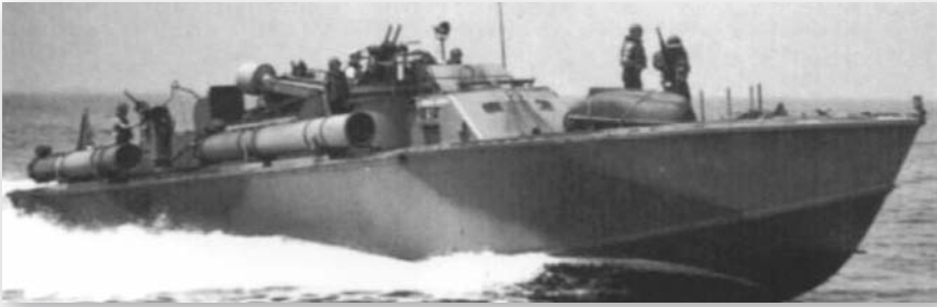
An 80ft Elco at moderate speed. A 6ft wooden dinghy, obtained by many boats for boat to shore movement, is on the forecastle. The SO radar mast is folded down to reduce the boat's profile.
