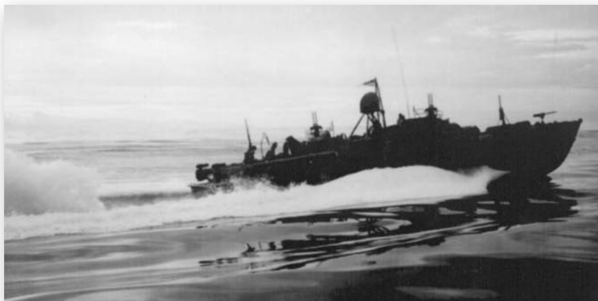
An 80ft Elco sets out on a night patrol off of New Guinea. Two .50-cals have been mounted on the forecastle.
