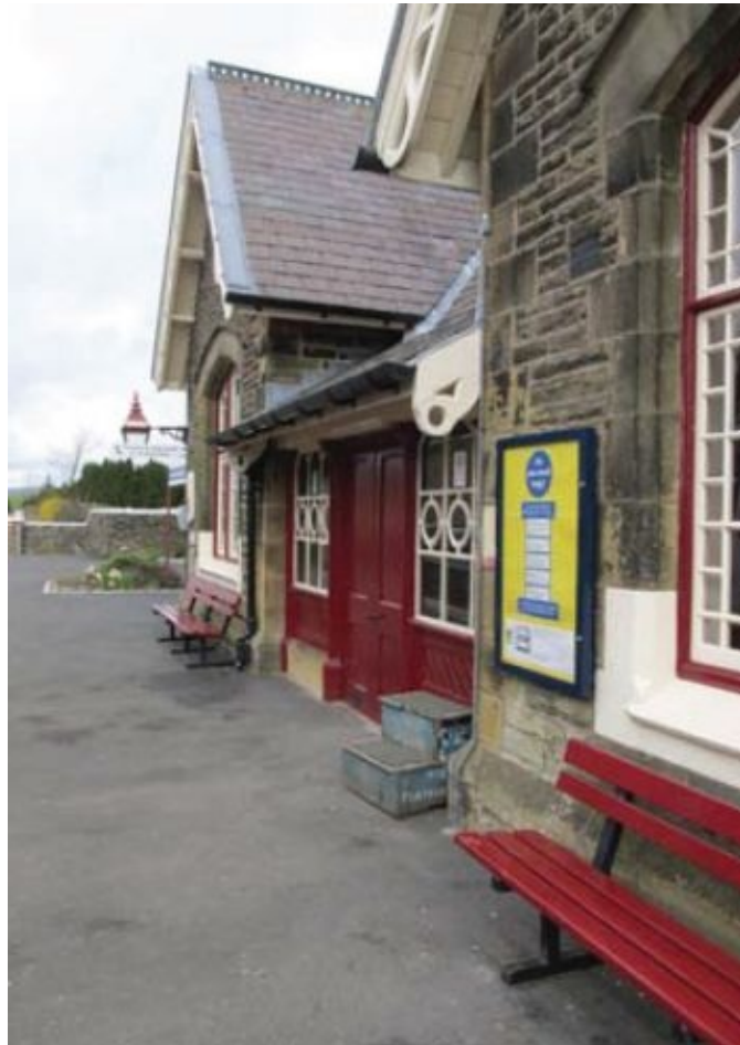
Horton-in-Ribblesdale typifies the Midland's Settle & Carlisle line. Note the portable steps, traditionally used at stations with low platforms.
