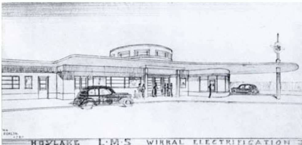
Hoylake: sketch by its architect, William Henry Hamlyn, highlighting the canopy wrapped round a totem pole and the circular clerestory of the booking hall.
