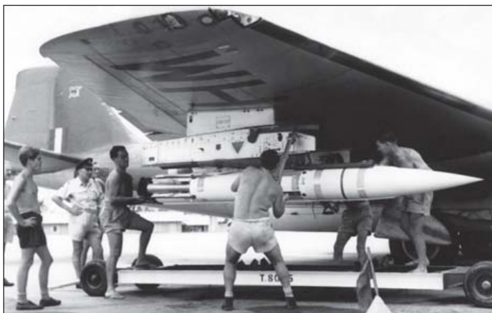
A French-built Nord AS.30 air-to-surface missile is loaded onto Canberra B 15 WH961 at Labuan. The post-Confrontation 'flying camel badge' is visible on the aircraft's fin (via Jefford)
