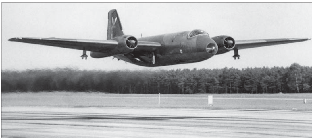
Eric Tilsley tucks the gear up but keeps the nose down in his No 213 Sqn Canberra B(I) 6 as he takes off from Brüggen in early 1969 – the unit disbanded in December of that same year. Single stores pylons, capable of carrying a 1000-lb bomb apiece, are clearly visible under each wing. (Peter Green Collection)
