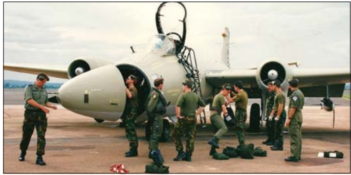
Film canisters are removed from XH169 at Entebbe in December 1996, the jet having completed yet another Rwanda flight. BOZ-107 chaff/flare dispenser pods can be seen on each of the underlying stores pylons (HQ STC)
