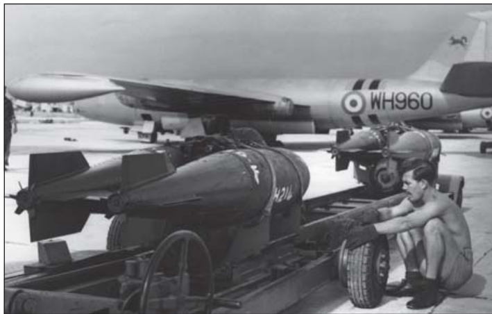
Getting ready for Suez, Canberra B 6 WH960 of No 12 Sqn is bombed up at Hal Far, Malta, in October 1956. The standard Canberra internal 6000-lb warload comprised two 'triplets' of 1000-lb bombs. The fox marking on the fin of this aircraft was red in colour (Peter Green Collection)
