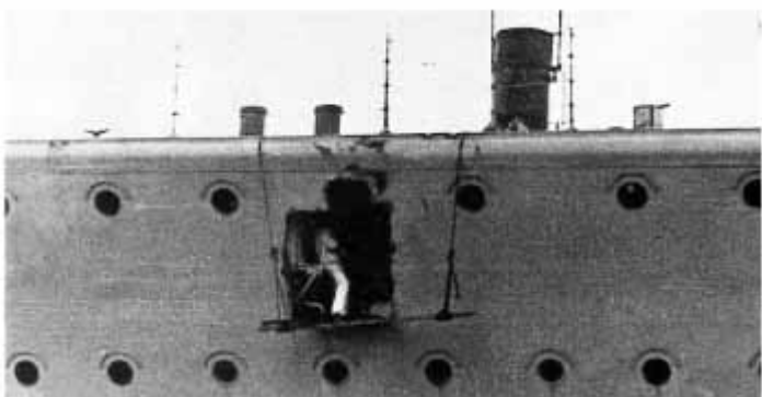
Temporary repairs to patch over a 6in hit in the port forecastle.
