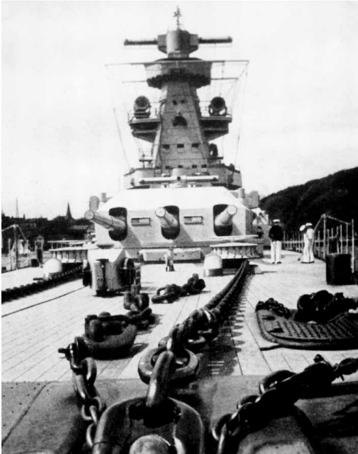
Looking astern over the anchor cluse near the forepeak towards 'A' turret and the battle-mast with its searchlights and bridge platforms. The chain of the second bow anchor is seen at the right.
