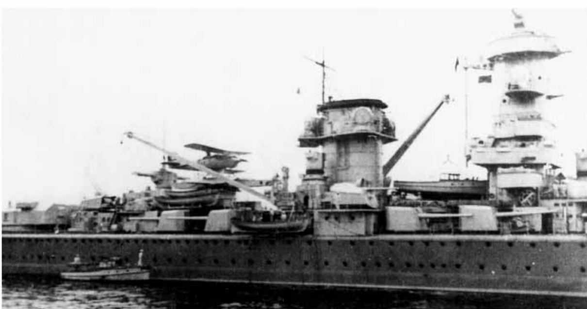
A midships view shows how the pole mast extended almost to the superstructure deck — twice the length of the fixture aboard Admiral Scheer . On the catapult is He 60 floatplane '60+F91'.
