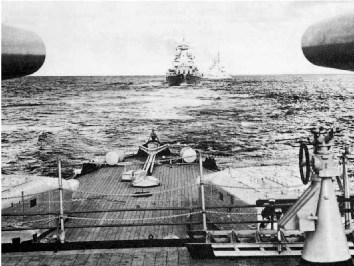
Admiral Scheer (nearest camera) and Gneisenau seen from Deutschland during the 1939 fleet gunnery exercises. Notice the lowered railing stanchions and ensign staff on the quarterdeck, the two smoke buoys and, in the right foreground, the mounting for a 2cm Flak gun, the weapon having been unshipped for protection from the elements.
