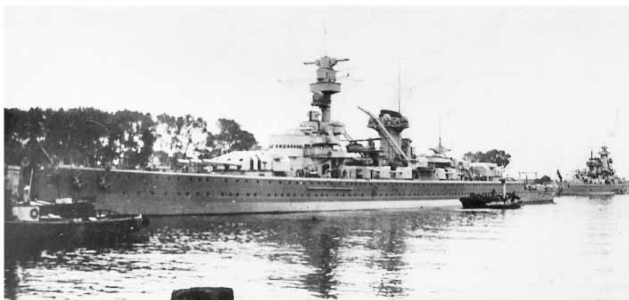
The bomb damage was quickly repaired and Deutschland , seen here at the Wilhelmshaven fitting-out quay with Admiral Scheer nearby, soon reported fully operational. Notice the new shipboard cranes and raked funnel cap.
