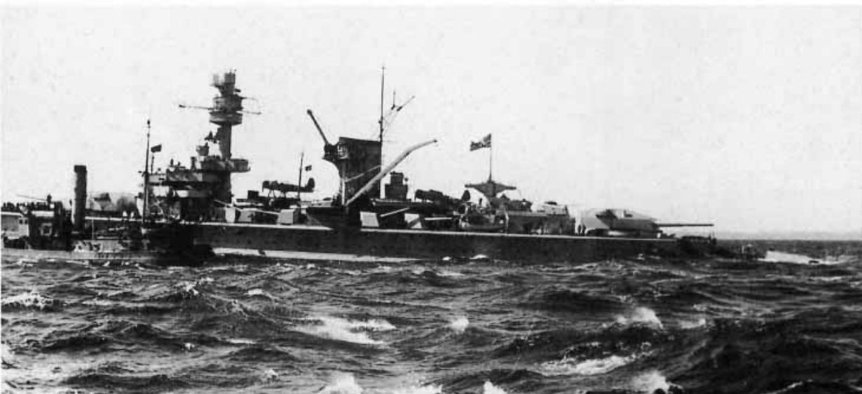
The cruiser seen from off the port beam. Her stern has been almost snapped off abaft the rear of the forecastle deck and is fully submerged save for the top of the torpedo tube sets breaking surface. Alongside a UJ-boat gives close antisubmarine escort. Note the Arado 196 floatplane on the catapult. This type replaced the Heinkel 60 at the outbreak of war.
