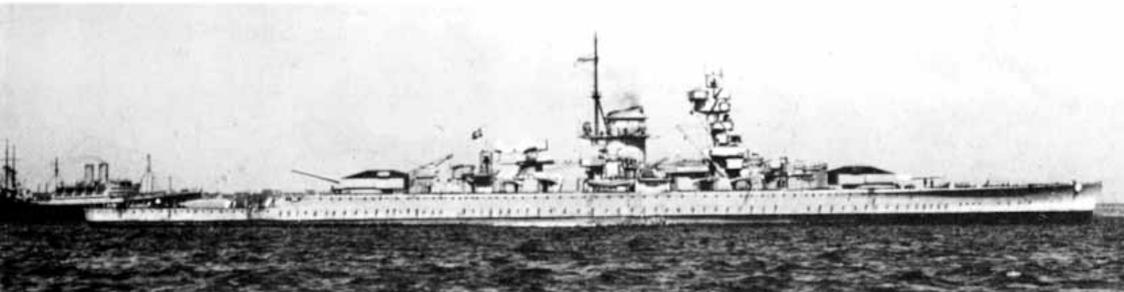
The new foretop, showing the 10.5cm rangefinder, single searchlight and forward Flak control centre.
