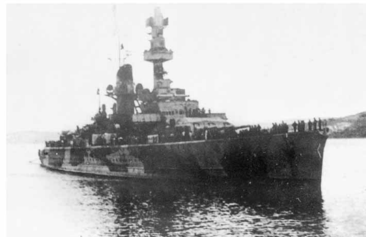
Lützow in late 1944, with FuMO and FuMB radar antennas at the foretop.
