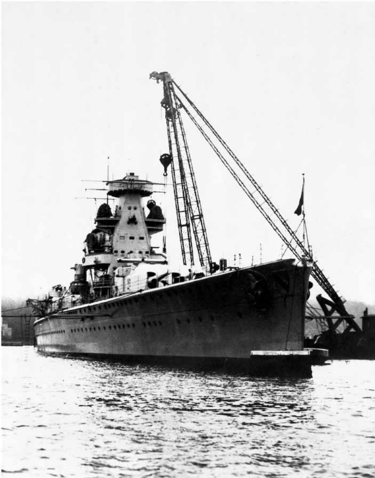
At moorings, Kiel, January 1935. A floating crane is alongside, probably for the installation of heavy gear. The foretop 10.5cm rangefinder has not yet been fitted.
