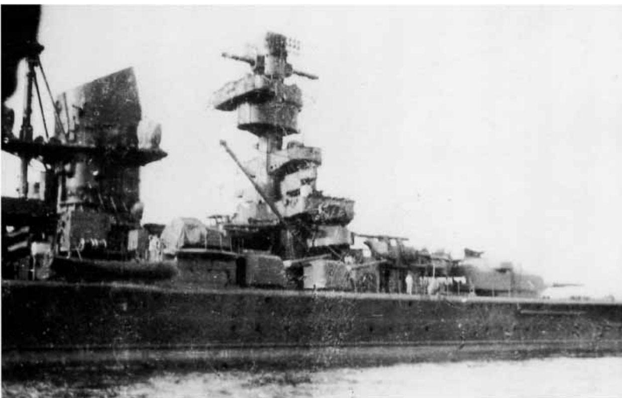
Two further photographs of Admiral Scheer in 1944–45, showing the large (2 x 6m) radar aerials at the foretop and after command centre.
