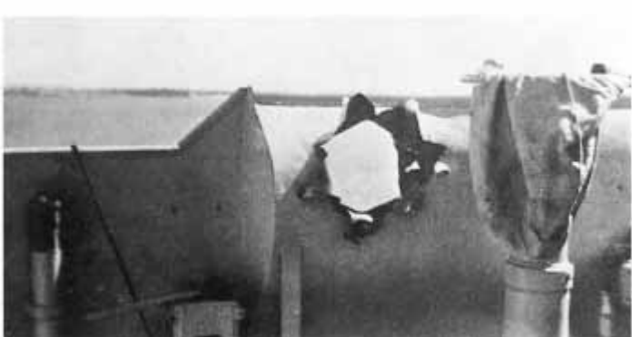
An 8in shell passed through the coaming of the admiral's bridge.
