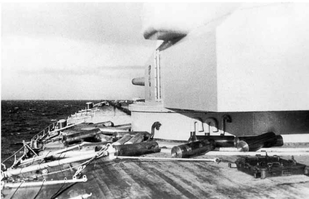
The aftermath of gunnery practice for the main armament: 'A' turret is at rest and numerous shell cases are strewn around the upper deck. The railing stanchions were lowered whenever the guns were in action.
