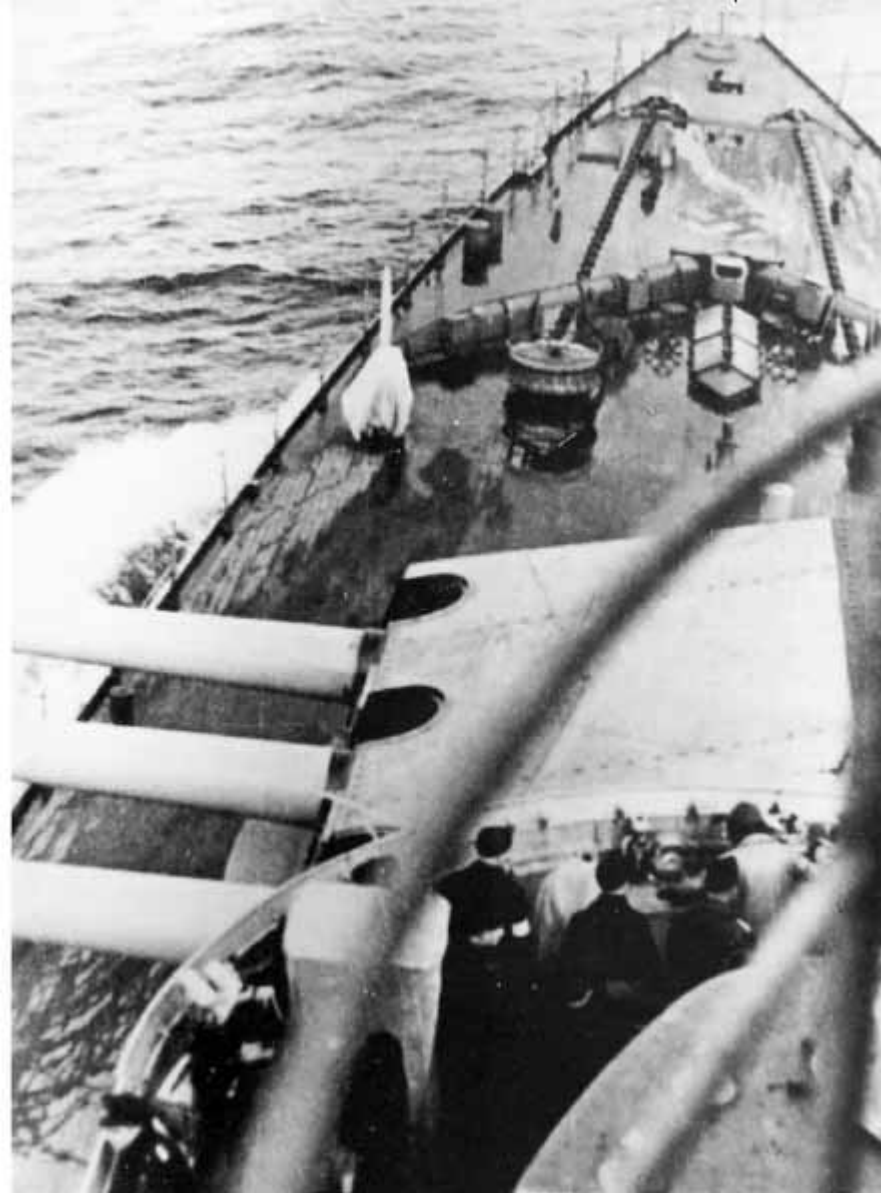
A view over the bow from the bridge, during operations in the East. Note the 2cm Flak gun under a tarpaulin abaft the breakwater. 'A' turret is trained to port.
