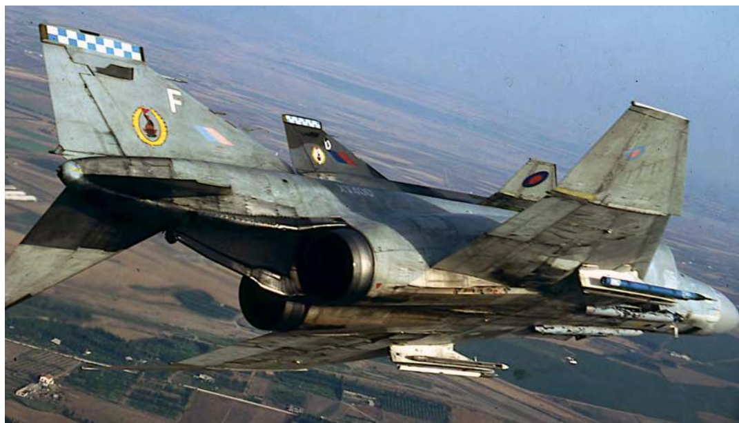
▲ Two 19 Squadron Phantom FGR.2s (XV400/F and XV468/D) on a training sortie, during the transition period between tactical pattern camouflage and low-vis grey scheme; note the ballast rounds in the forward Sparrow bays, ACMI pod on the starboard inner and AIM-9 acquisition missile on the port inner wing pylon. (Ian Black)
