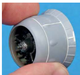
▲ The gap in the cowls was for a vent not present on Mk.I Benheims, so it was filled with plastic card and strip.
