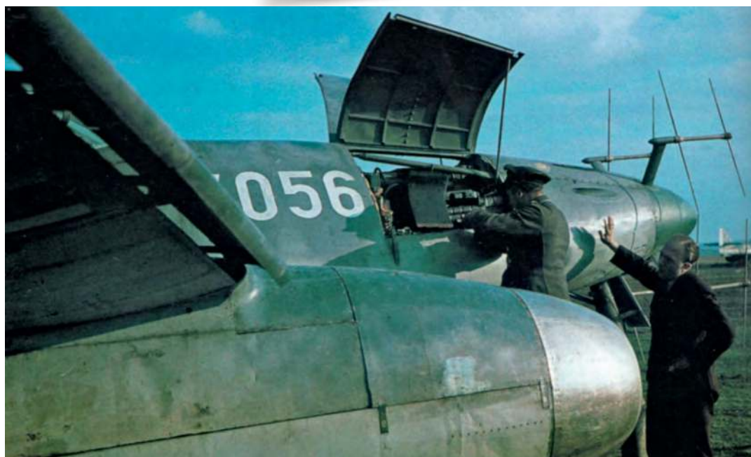
This single-seat Me 262 prototype/development aircraft V056 was used in trials to determine the best arrangement of nose-mounted aerials for the FuG 218 Neptun radar, as used in the Me 262B-1a/U1 night fighter. (Peter Walter Collection)
