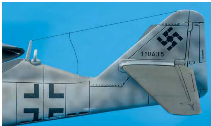
▲ The aircraft wire antenna was fashioned from Uschi van der Rosten elastic line, secured with CA.
