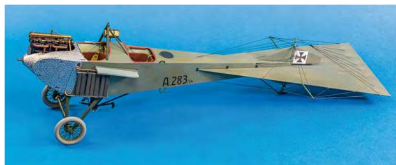
▲ Aside from the propeller and windscreen, the Stahltaube's fuselage was rigged and finished before the wings were added.
