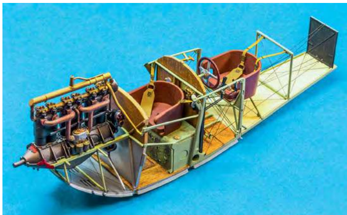
▲ The finished cockpit and engine insert revealed the lengths Wingnut Wings had gone to, in reproducing the Stahltaube's interior faithfully.
