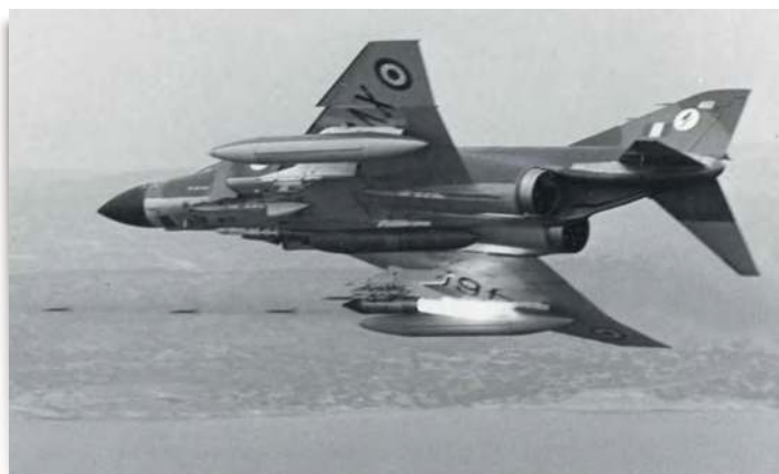
▲ Down on the range. An early 6 Squadron FGR.2 (possibly XV461) fires 68mm rockets at a target. It's also equipped with practice bombs, a centreline gun pod, strike camera and Sparrow training round.
