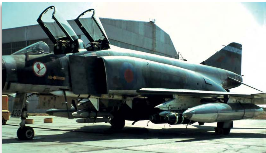
▲ How's this for modelling inspiration? Phantom FGR.2 XV420/H wears 6 Squadron markings and is loaded with Lepus flares, BL755 cluster munitions, AIM-7E2 Sparrows and a centreline gun pod.
