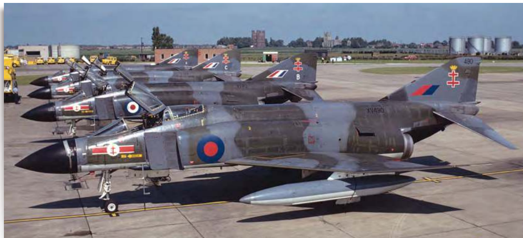
▲ One for fans of weathering; this line-up of 41(F) Squadron FGR.2s highlights the retouched paintwork along panel joins, with matt, rather than the original gloss paint employed. (Denis J Calvert/I-AP)
