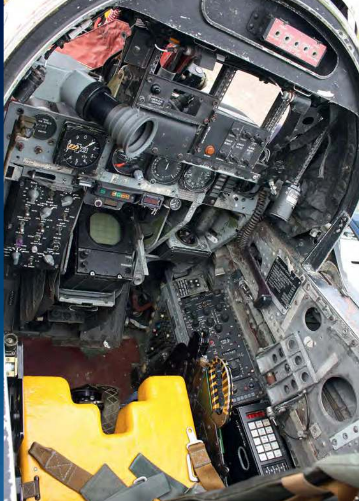
▲ The navigator's cockpit in the Phantom FGR.2. Note how cluttered the instruments are, and the periscope on the left-hand side; otherwise the rear crewman had little, if any, forward vision.
