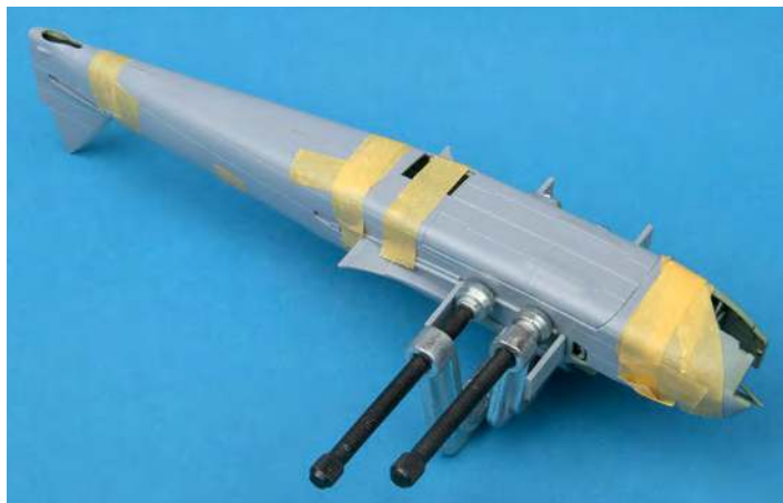
▲ Fit was tight around the bomb bay, so clamps were brought into play, to assist while the glue dried.
