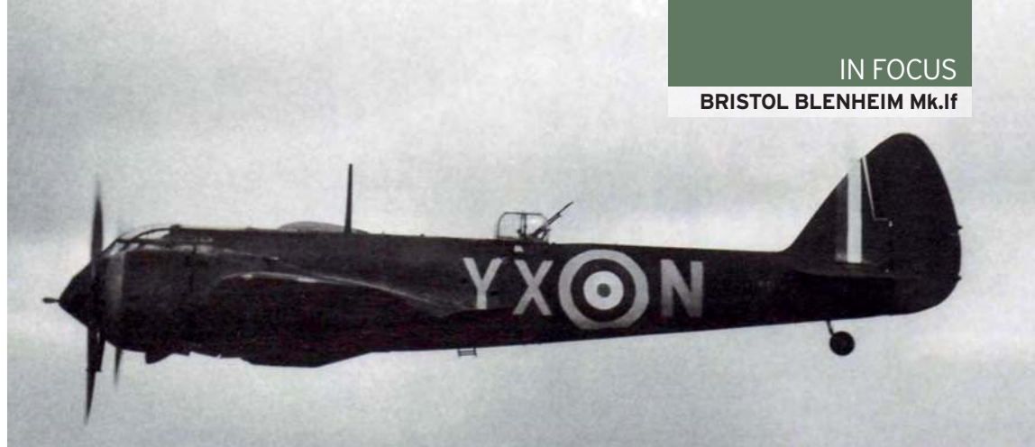
The functional lines of the Blenheim Mk.If are obvious in this image of YX-N/ K7159 from the training unit 54 OTU. The partially streamlined gun pack can be seen attached to the lower fuselage. (All Malcolm V Lowe Collection unless stated)
