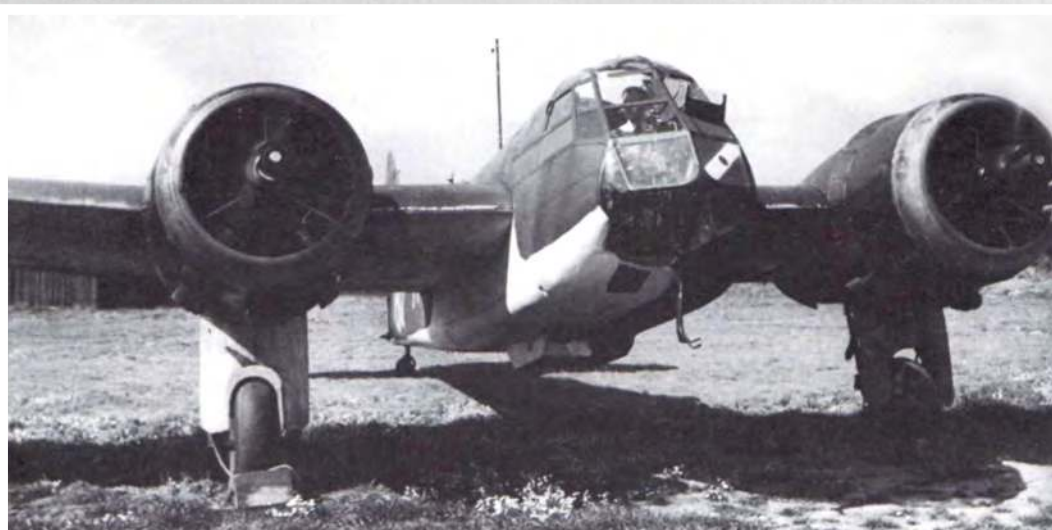
The configuration of the gun pack beneath the fuselage of the Blenheim Mk.If is evident in this view, although the four .303in Brownings aren't installed. Some Blenheim Fighters were initially delivered without the gun pack fitted.
