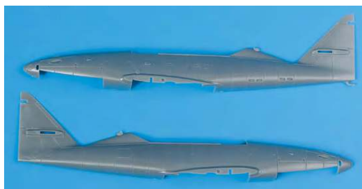
▲ The Me 262B fuselage differs considerably from the single-seat version, with a much-lengthened cockpit and raised fairing ahead of the tail for the canopy.
